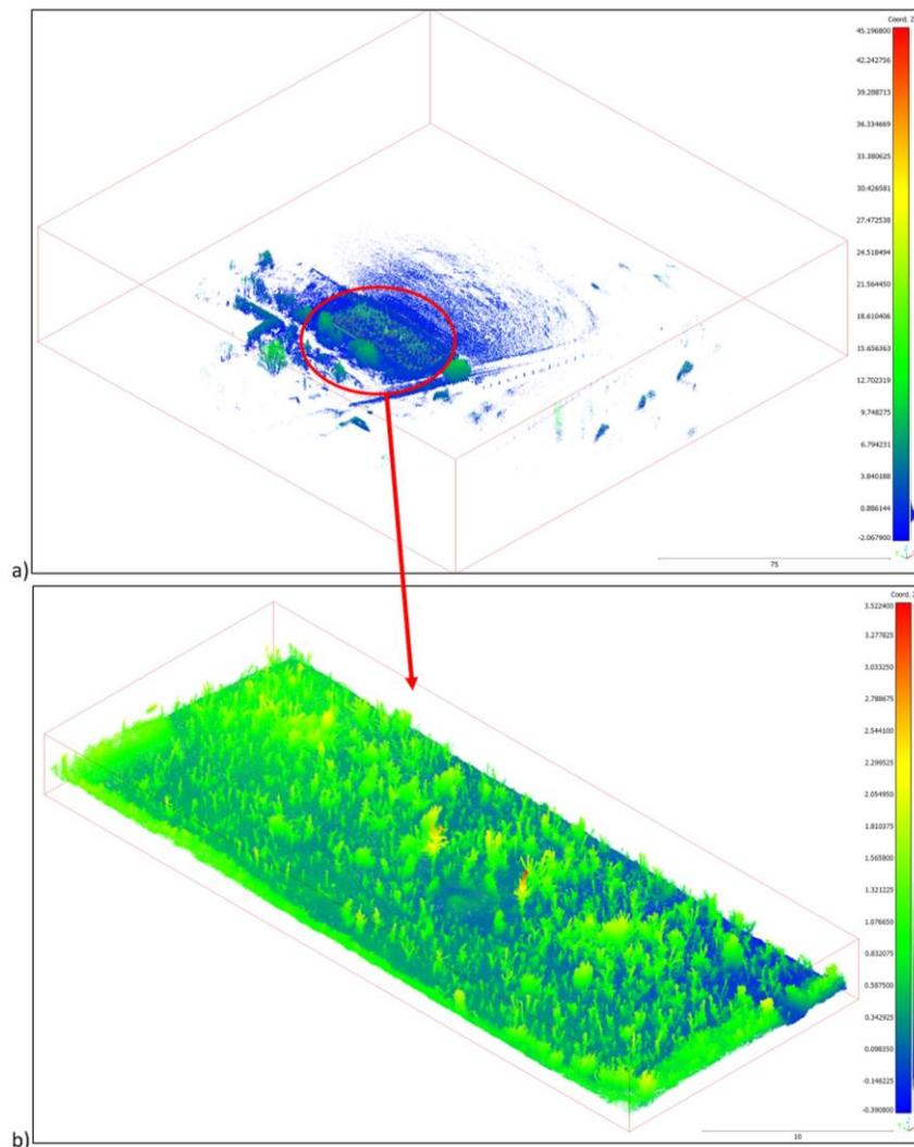
6: a) Point cloud before clipping at 75 m scale in Cloud Compare b) Point Cloud after clipping to 17 m x 43.5 m
