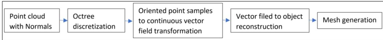
Normals of each dataset were computed with a 'quadric' surface approximation, good for curvy surfaces, within a 1cm radius neighbors and +Z axis orientation. Poisson Surface Reconstruction was applied to the each dataset with "Dirichlet" border structure, resulting in more accurate model (Michael Kazhdan, 2020), 12 level octree dept were choosen.
