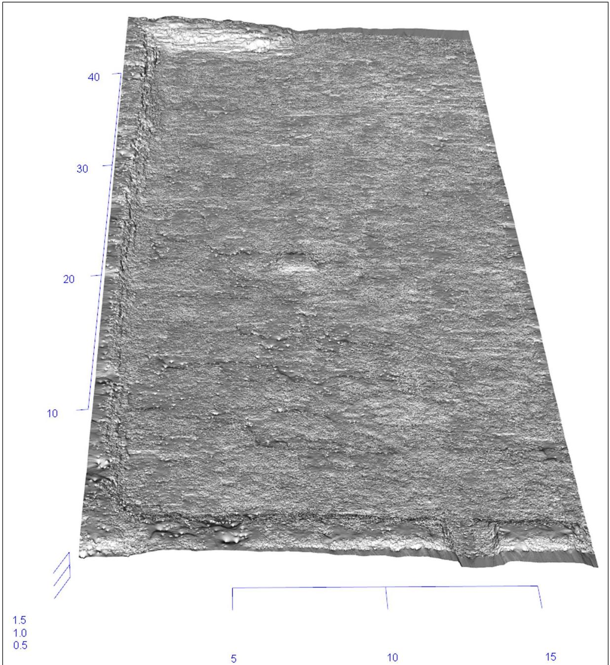
13: Creating Digital Terrain Model of Tiny Forest using inverse distance weighting (IDW) interpolation with 1 cm resolution in RStudio, front view.
