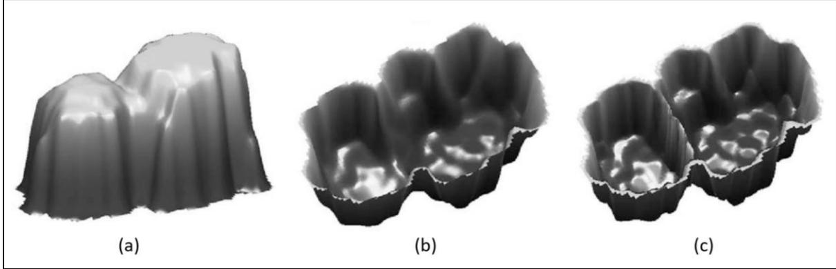
8: An illustration of watershed segmentation Algorithm. (a) A CMM, (b) the complement of the CMM, and (c) dams built at the divide line (Chen, 2006).
