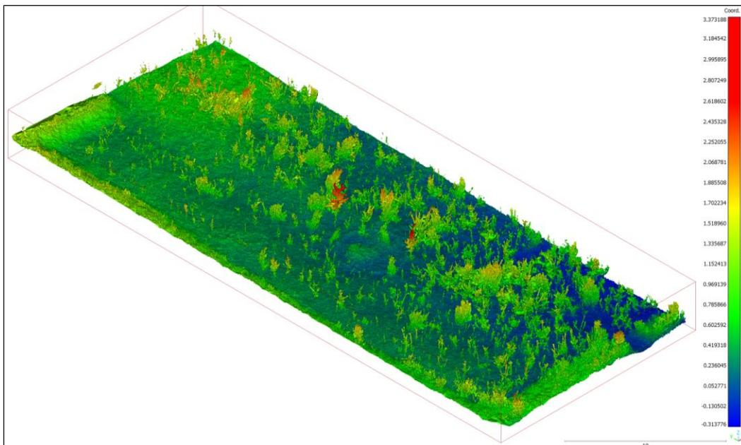
11: b) Poisson Surface Reconstruction of the merging of 'interpolated ground points' and 'off-ground points'
